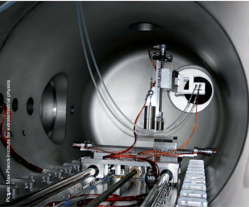
Motorised multi-axis mechanism inside an ultra high vacuum chamber.
